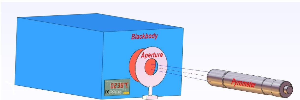
The first official calibration geometry formula for nominal distance "a" and spot size "M" gives the necessary radiation source aperture "A" when calibrated at the calibration distance "a":
